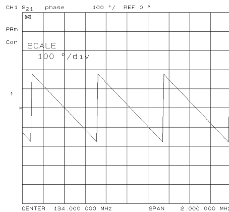
Figure 2-29. Linearly Changing Phase
